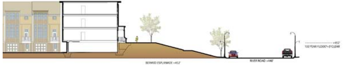
100 year protection for the 60 acres should be achieved by lifting any habitable spaces above the flood level. Parking can be placed below in a floodable zone. A landscaped earthen berm would be the preferred method of screening.
