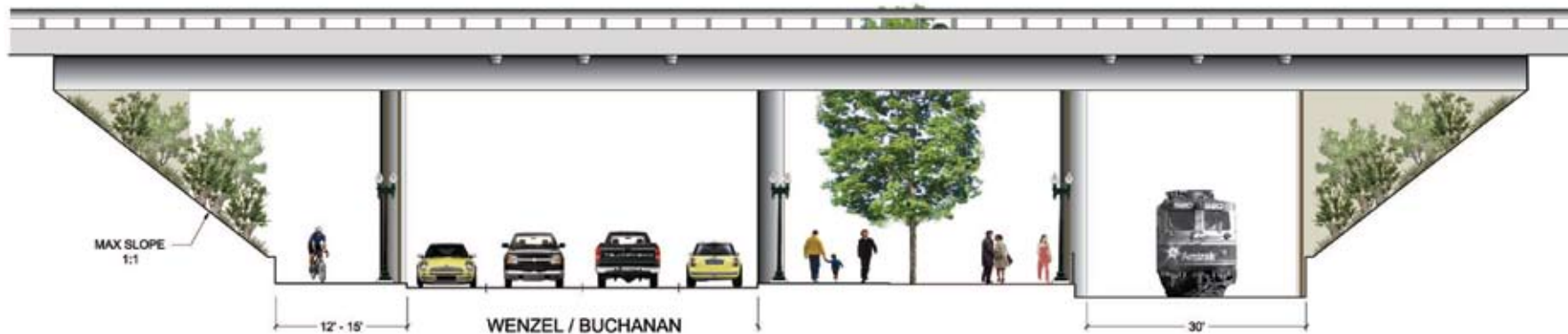
Schematic street section at Wenzel/Buchanan Street underpass. Swinging flood gates can be installed below the interstate bridges to provide flood protection for Butchertown.
